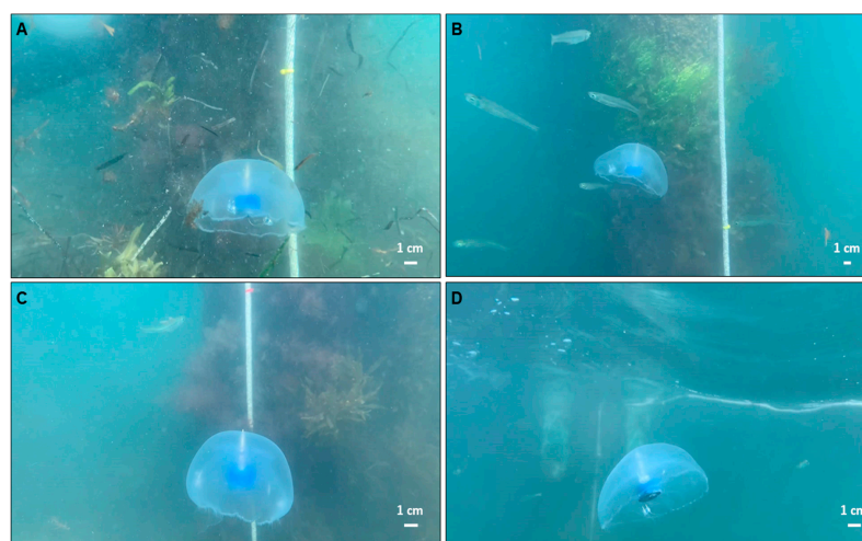
Figure 3. Representative images of biohybrid robotic jellyfish during field experiments. Examples of one biohybrid robotic jellyfish (animal 1) (A) initiated at the ocean bed and stimulated at 0.50 Hz, (B) swimming toward the ocean surface at 0.50 Hz, (C) initiated at the ocean bed and stimulated at 0.50 Hz (second trial), and (D) swimming toward the ocean surface at 0.50 Hz (second trial).
